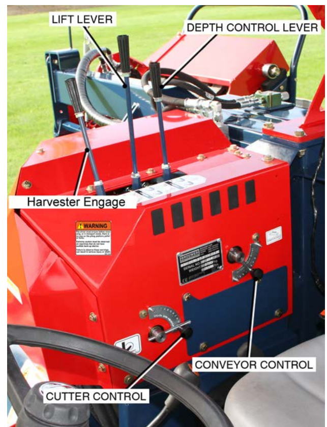
Cutter Knife Speed, Conveyor Speed Controls Cutter Head, Lift and Depth Control Levers
