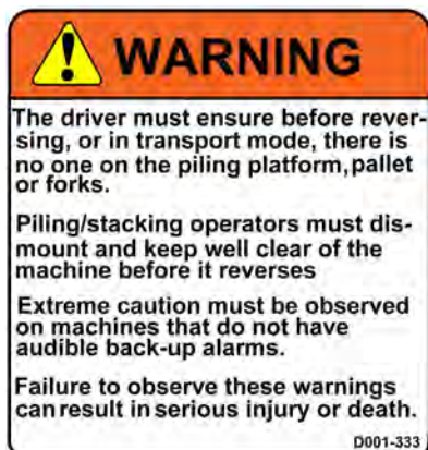
Location: Rear Cross Beam.
