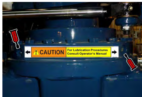
Slewing Ring. Lubricate in four places.
