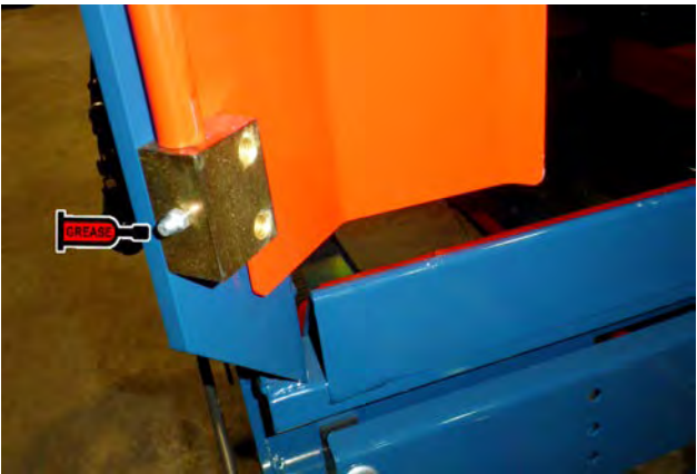
Pallet Retainer Flap. (Two Places. Bottom shown).
