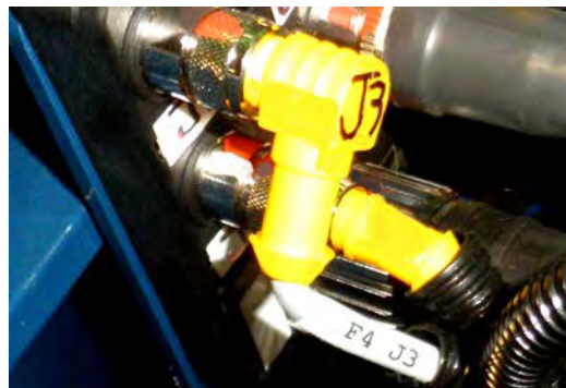
Cable Identification. Front 4-Port Block. Port J3.
