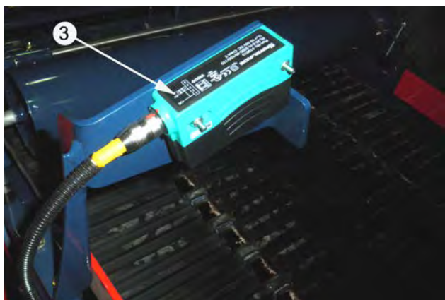
3. Electronic Sod End Sensor. (See page 4-24 for mechanical (PROX) sensor).
