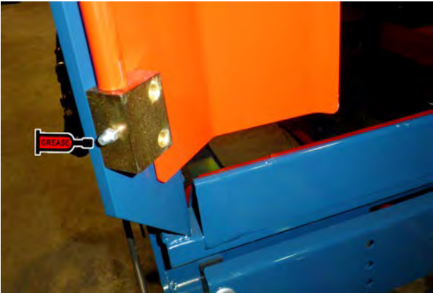
Pallet Retainer Flap. (Two Places. Bottom shown).
