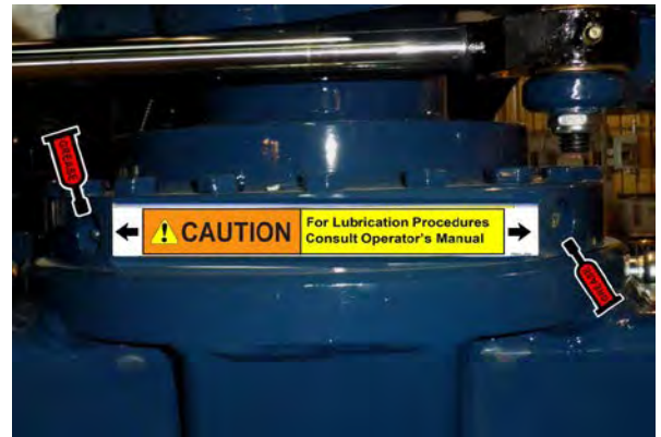
Slewing Ring. Lubricate in four places.
