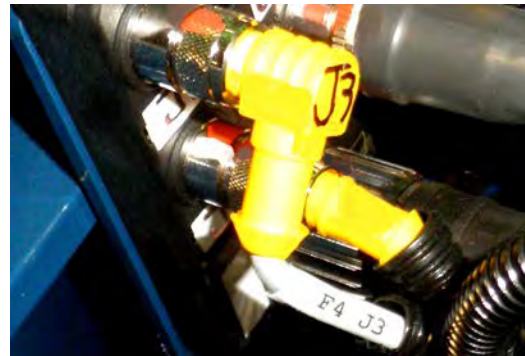
Cable Identification. Front 4-Port Block. Port J3.
