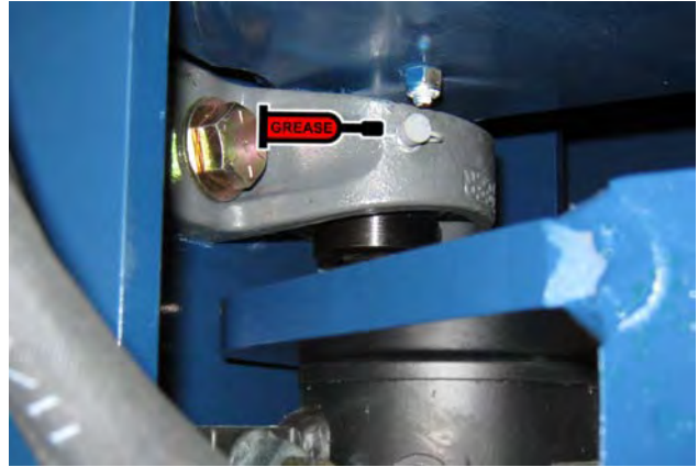
Pallet Injector. Lower Pivot Bearing.
