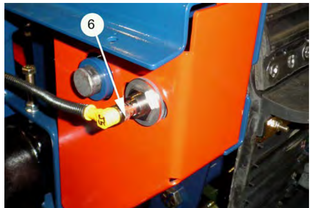
6. Index Conveyor 'CLEATS' Position Sensor.
